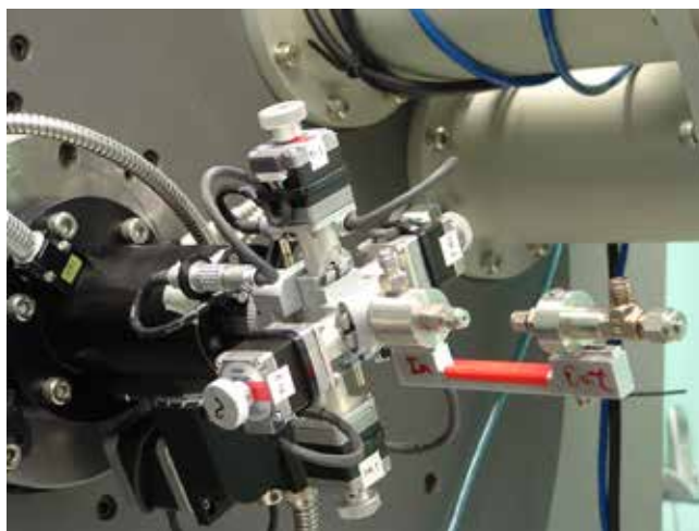
Figure 4: Gas flow through cell at the Powder Diffraction beamline for determination of the structures of hydrogen storage materials.
