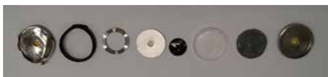
Figure 3: An example of the contents of a battery cell used for in situ cycling
