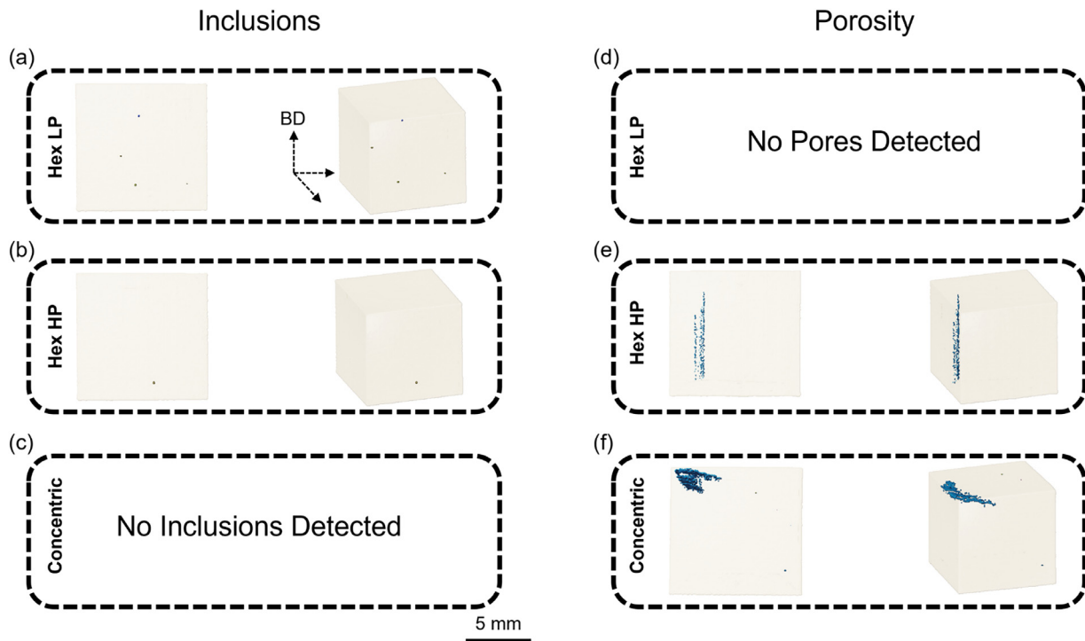
Fig. 12. Results of neutron computed tomography. Detected inclusions are shown for (a) Hex LP, (b) Hex HP, (c) Concentric samples. Detected pores are shown for (d) Hex LP, (e) Hex HP and (f) Concentric samples. Note that each panel shows two different views of the same data.
