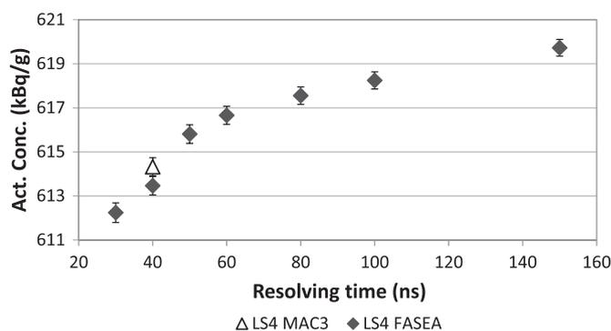
Fig. 6. Effect of variation of resolving time on the result of one source measured with the MAC3 and FASEA data acquisition systems. Data was collected with the MAC3 (unshaded triangle) at a fixed resolving time of 40 ns, while the data collected with the FASEA system (grey diamonds) could be analysed for a range of resolving times. A resolving time of  $\tau_R = 60$  ns was applied for the final result. Error bars indicate statistical uncertainties at  $k = 1$ .
