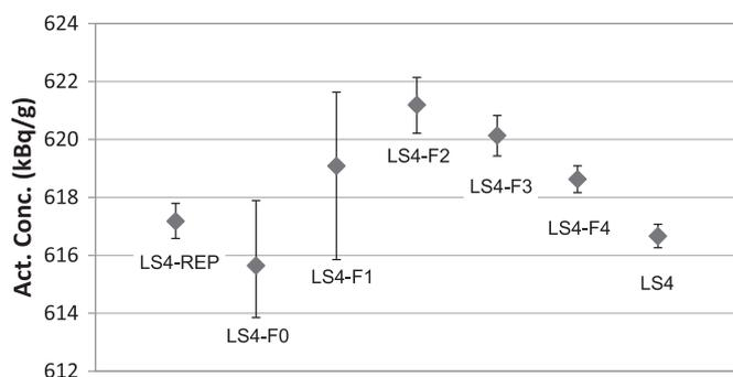
Fig. 5. Results of one source measured without (LS4 and LS4-REP) and with grey filters of increasing light absorption (LS4-F0 to LS4-F4). Variation in the extracted activity concentration indicates some inconsistency in the efficiency calculation model, which was incorporated into the uncertainty budget (Table 2). Only the data from sources counted without grey filters were used to calculate the final activity value. Error bars indicate statistical uncertainties at  $k = 1$ .
