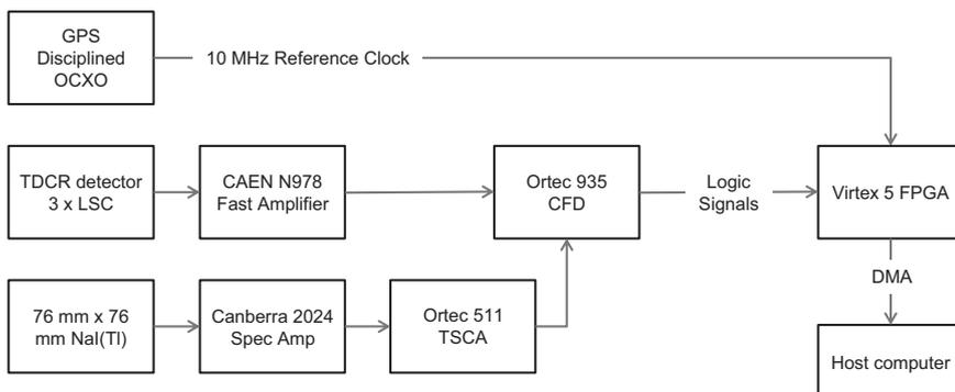
Fig. 2. Schematic diagram of the detection system used for data acquisition (Steele, 2009).
