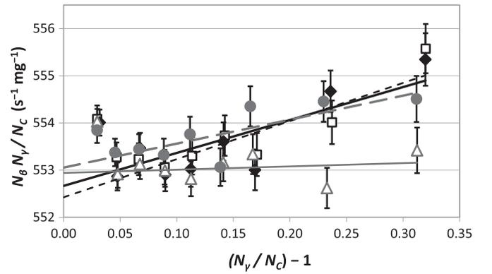
Fig. 3. Plot of weighted linear regression to the eight lowest efficiency points for each of four sources. Error bars indicate statistical uncertainties at  $k = 1$ . The highest efficiency points included some electron capture emission and these points were excluded from the regression.
