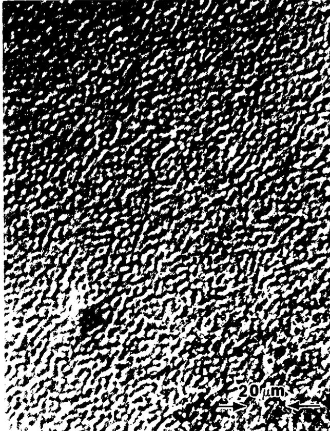
FIGURE 1. THE SLIGHTLY EXAGGERATED 'ORANGE PEEL' FINISH FOUND ON AN Si SAMPLE AFTER PULSED LASER IRRADIATION
