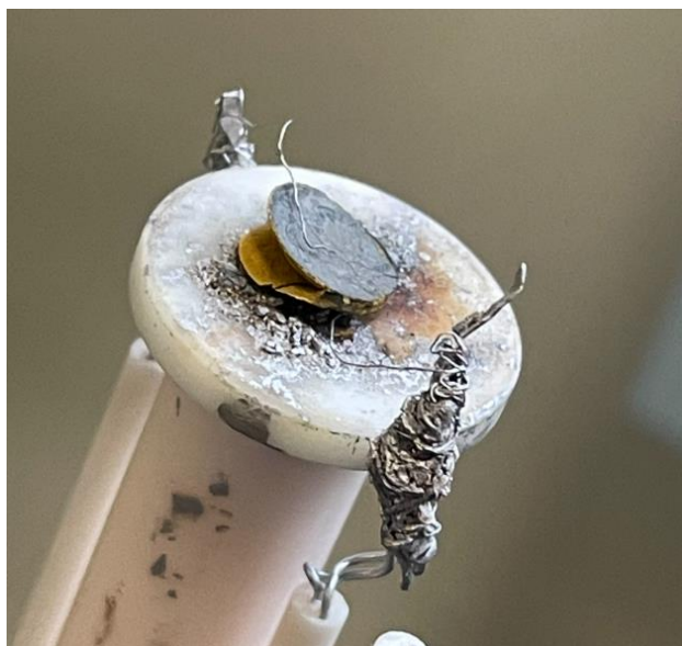
Figure S21: Mounted pellet of \text{Ba}_5\text{Tb}_2\text{Al}_2\text{SnO}_{13} after conductivity measurement in wet \text{N}_2 , showing that the pellet has cracked in half due to significant decomposition.
