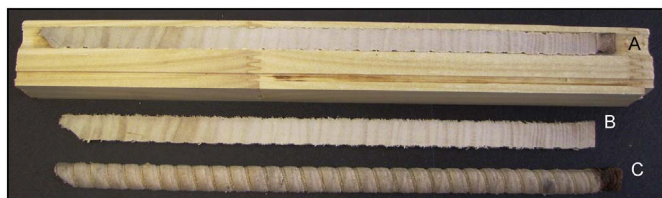
Fig. 3. Sample DMA026E after being cut with a twin-bladed saw. Each core is comprised of A) the bottom section of the core which is glued into the base, B) a lath of 2 mm depth for scanning on the Itrax core scanner, and C) the remaining portion of the core which can be used for destructive analysis such as radiocarbon dating. While some evidence of ring boundaries are present in the DMA samples there are large parts of the cores where such boundaries cannot be identified as evidenced by the central portion of DMA026E.
