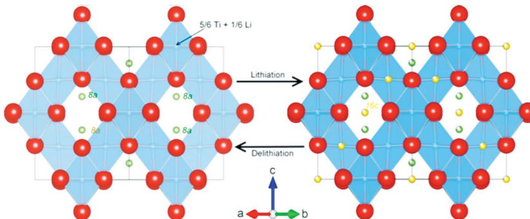
Figure 1. (Color online) (Left) Crystal structure of the as-prepared  $\text{Li}_4\text{Ti}_5\text{O}_{12}$  as refined using high-resolution NPD data. Li (8a) is shown in green, O in red, and mixed Ti/Li sites in light blue. For clarity, Li and Ti sites are shown as fully occupied. Li at 16c sites (yellow) are also shown in the  $\text{Li}_{4+z}\text{Ti}_5\text{O}_{12}$  structure (right) following lithiation.
