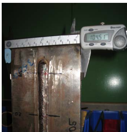
First weld scanned on Kowari, June 2008: the scan was done along the transverse direction (perpendicular to the weld) at the centreline indicated on the plate.
