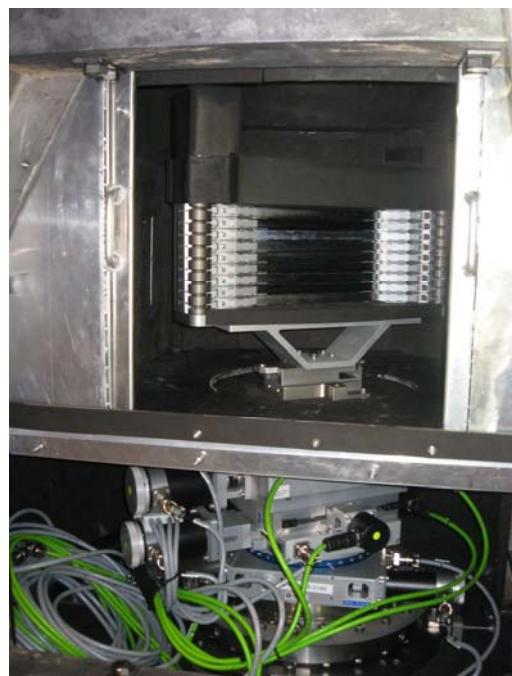
A load frame for tension, compression and fatigue testing of samples on Kowari has recently been tested, see photo below, at the manufacturer Instron (High Wycombe, UK) and will be shipped at the end of April. This
