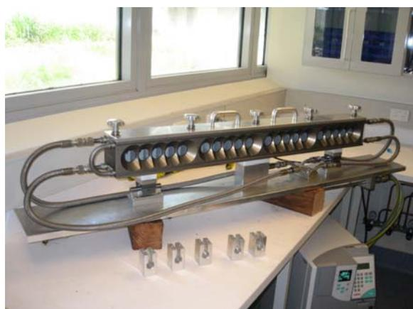
Based on a design at the NIST facility (National Institute of Standards and Technology, Centre for Neutron Research) in the USA, a 20-position sample changer, heated and cooled via a Julabo water bath, has begun acceptance testing. It should be available as Quokka comes on-line in mid 2007. Additional information on the sample environment ancillary equipment at Bragg can be found at <http://www.ansto.gov.au/ansto/bragg/ancillaries/index.html>.
