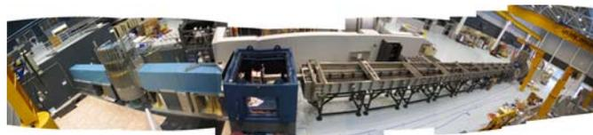
Quokka at full length in early February during the guide installation in the collimation section (before shielding tunnel placement).
