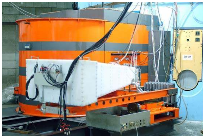
FIG. 1. The IPEN-CNEN/SP PSD Neutron Powder Diffractometer. (Photo by Marcello Vitorino).
