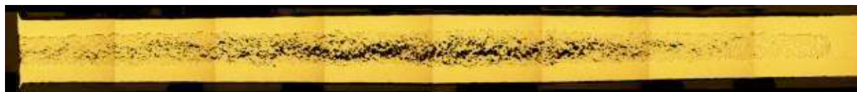
Fig.1: FUTURE metallography in the pillowed region (plate transverse section)
