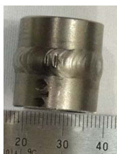
Figure 12. Photograph of the steel pipe weld used in the experiment.
