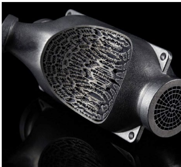
Figure 3.4: 3D synchrotron X-ray Computed Tomography: non-destructive imaging of complex additive manufactured components.
