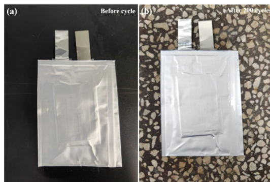
Figure S18 Optical images of the (Nb, Mo)13O33 containing pouch cell before and after 200 charge/discharge cycles.
