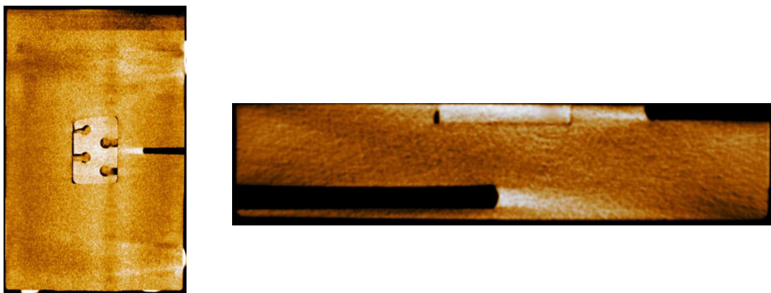
Figure 4 slice through 3D model of reconstructed copper tungsten sample
