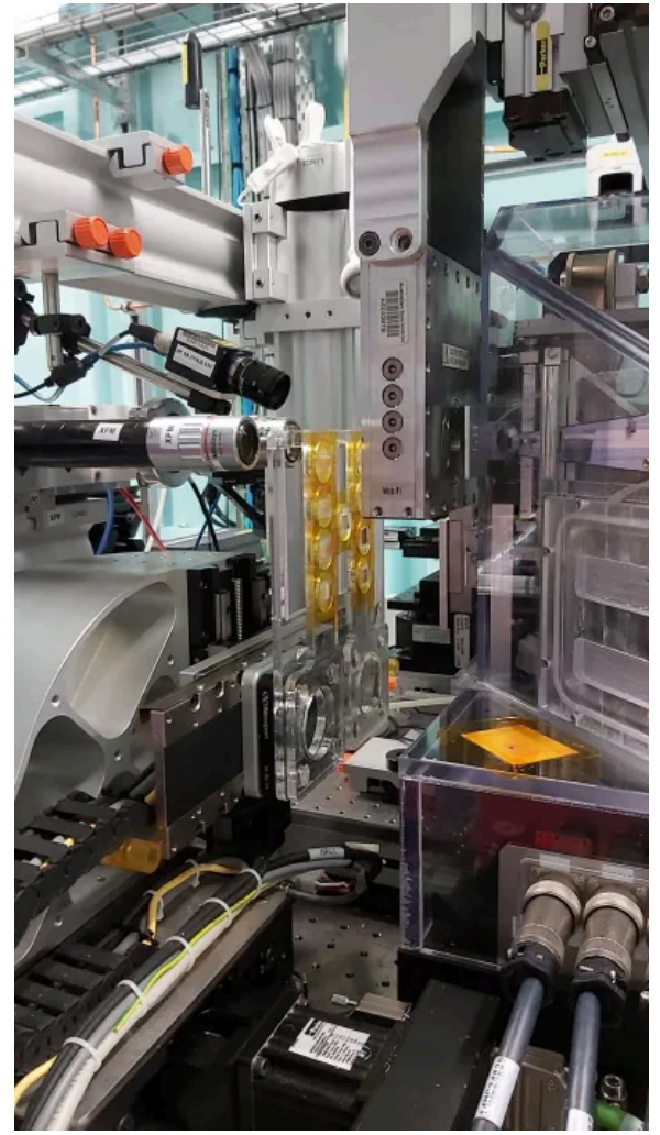
Stalagmite samples mounted and ready for analysis at the Australian Synchrotron XFM beamline. Credit: Micheline Campbell
