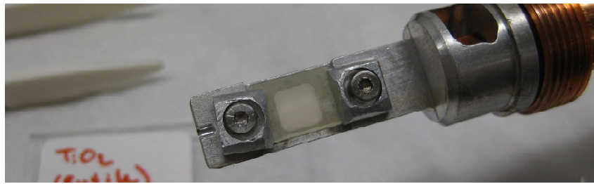
Figure 1. Cleaved rutile \text{TiO}_2 (100) substrate from Crystal GmbH mounted in the \beta -NMR sample holder. The pale yellow colour is indicative of a minor presence of defects.
