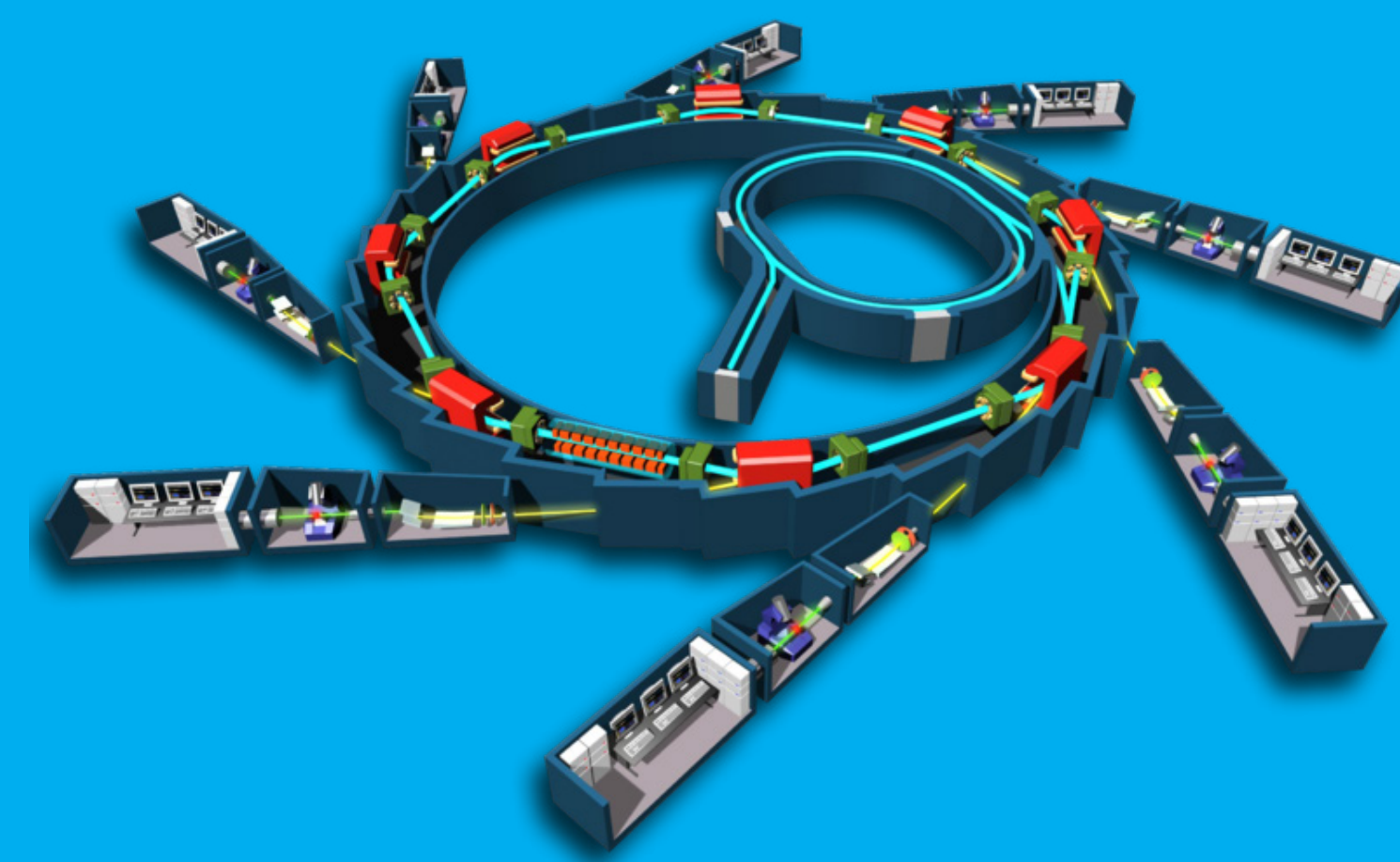
General diagram of a synchrotron. Copyright © Chris Wood at synchrotron, used with permission.
