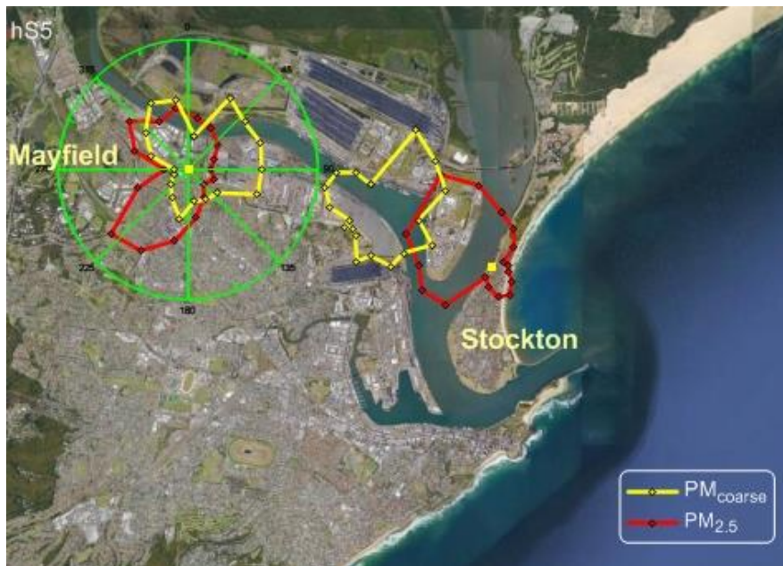
Figure 89: Fingerprints, CPF and time series plots of PM 2.5-10 Factor 5 (industry)
