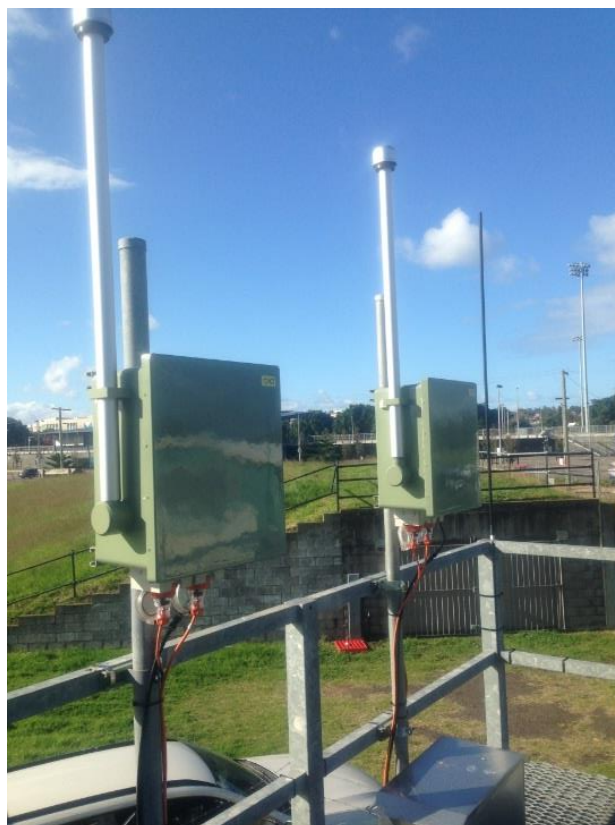
Figure 16: ASP samplers (Teflon filters on left and quartz filters on right) installed at the OEH Newcastle Air Quality Monitoring Station
