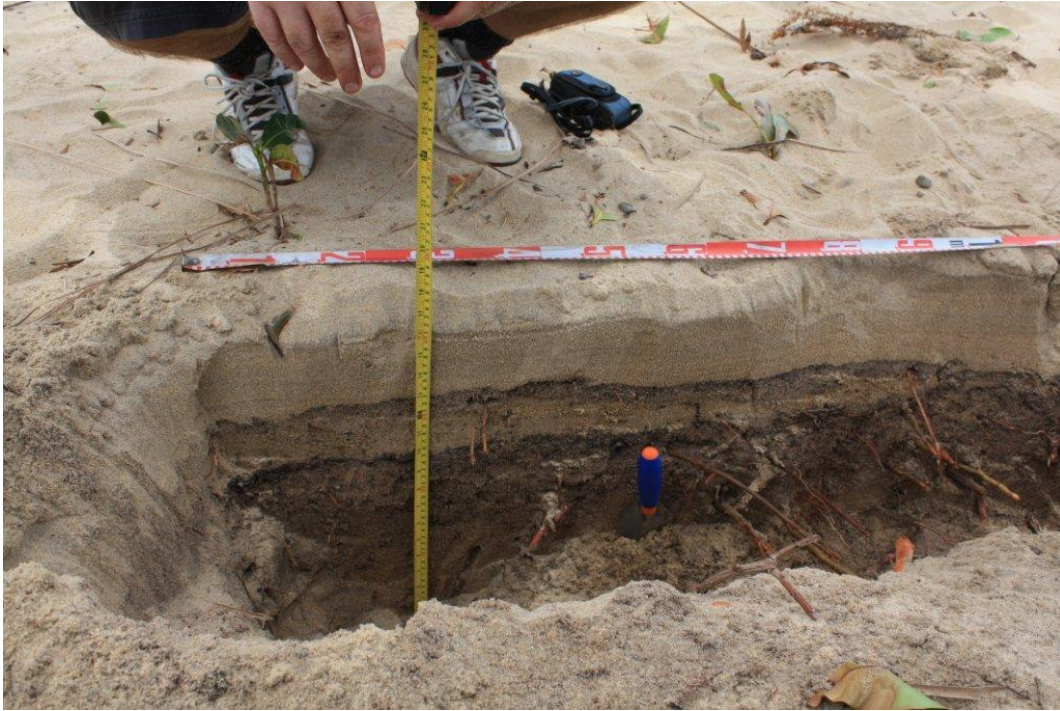
Figure 16: Cowley Beach – A second sand unit is visible about 2.40 m landward of the scarp eroded by TC Larry. This is the TC Larry deposit which is noticeably more weathered than the overlying sands of TC Yasi. The TC Larry sediments overlie another buried soil beneath which is a heavily weathered sand that we tentatively associate with the 1918 Innisfail cyclone (see Figure 17).
