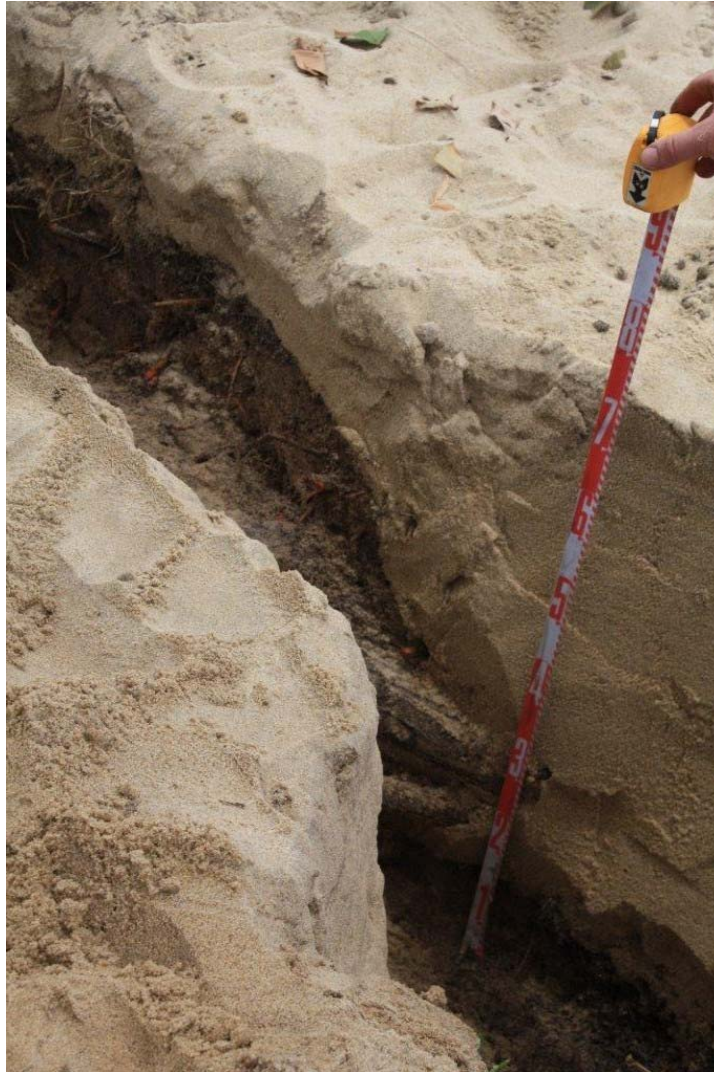
Figure 15: Cowley Beach – Pre TC Yasi scarp shown by the marked dip in the underlying soil. This marks the old erosional scarp of TC Larry.
