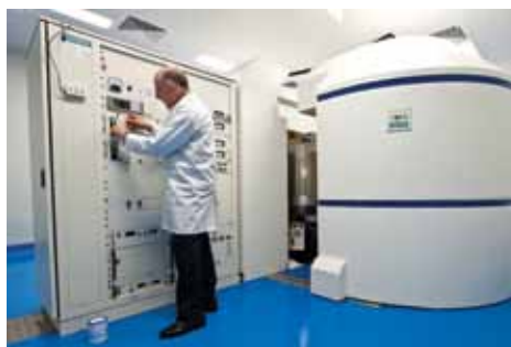
PETNET's twin mini-cyclotrons produce radiopharmaceuticals used in positron emission tomography (PET).
