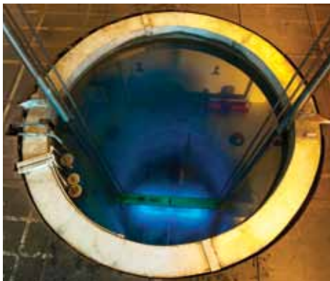
The GATRI pool. GATRI is a wet storage cobolt-60 batch irradiator.
