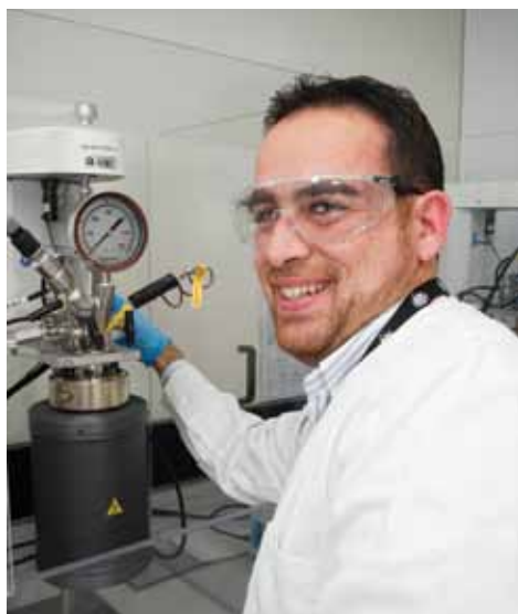
Tamim Darwish is setting up a hydrothermal deuteration reaction in a Parr high pressure reactor.
