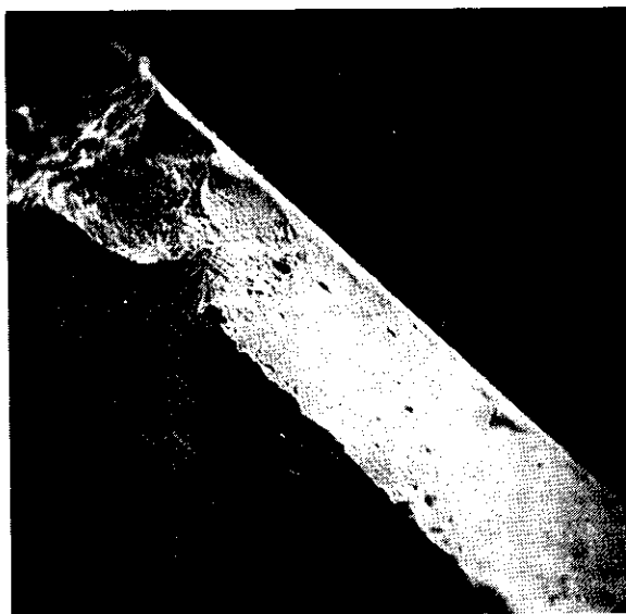
FIGURE 7 SHEAR FRACTURE AT 45° TO TENSILE AXIS ON 0.175 mm THICK SPECIMEN. 160 X.
