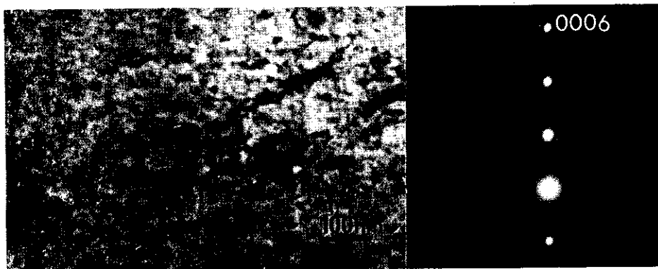
FIGURE 2 GROWN-IN \underline{c} COMPONENT DISLOCATIONS IMAGED IN \underline{g} = (0006) .
