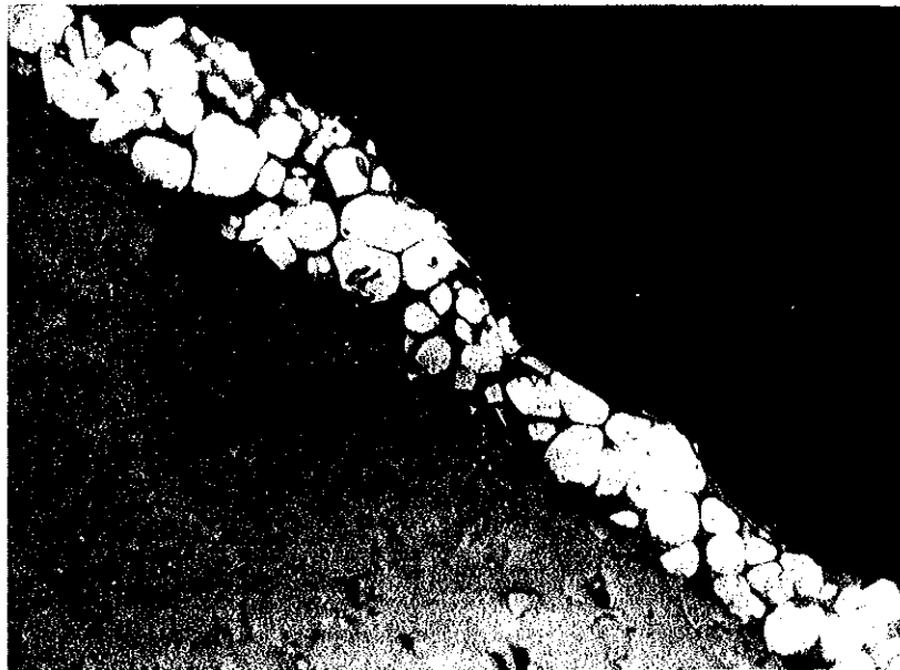
FIGURE 3 TYPICAL MICROSTRUCTURE OF A PREDOMINANTLY CRYSTALLINE GLAZE (GLAZE H, TABLE 1)
