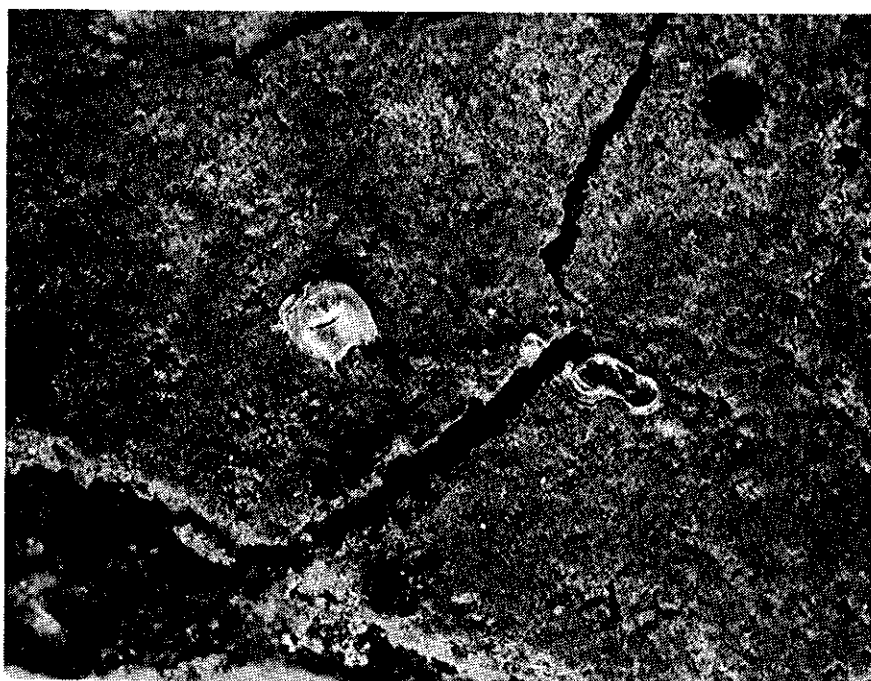
FIGURE 10. SPECIMEN D, SHOWING PLASTIC BUBBLES (AREA MARKED IN FIG. 8, ENLARGED \times 5.75 )
