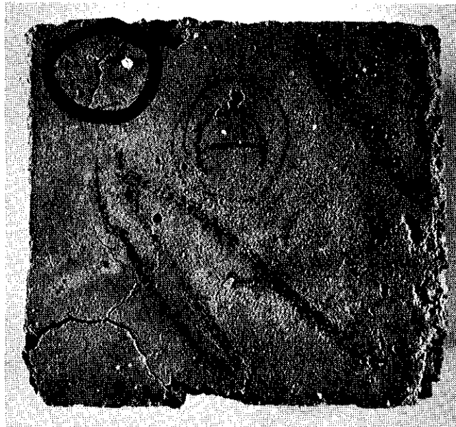
FIGURE 7. PMMA-CONCRETE COMPOSITE AFTER 93 h IMMERSION IN SATURATED LIMEWATER. SPECIMEN NOT DRIED BEFORE IMPREGNATION
