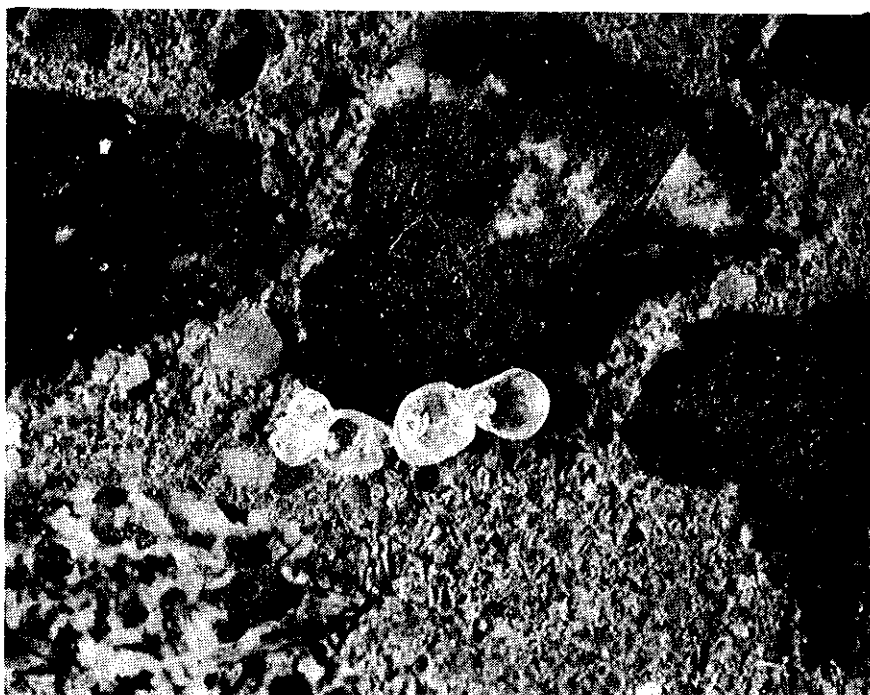
FIGURE 9. SPECIMEN B, SHOWING PLASTIC BUBBLES ( \times 5.75 )
