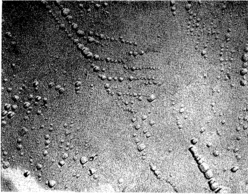
(a) Irradiated at pile temperature and annealed
