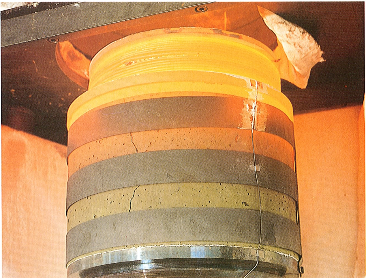
SYNROC filled bellows immediately after hot pressing at 1200 °C
