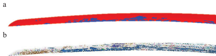
Fig. 2. a) A cut through the tomographic reconstruction of blade H1360; the red area is steel, while inclusions are colored in blue. b) 3D map of porosity rendered in false color.
