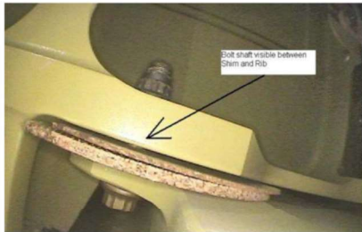
Figure 1. Bolt shaft can be seen through the gap between the shim and rib
