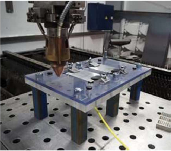
Figure 1. Test Samples Mounted in the RMIT Trumpf Laser
