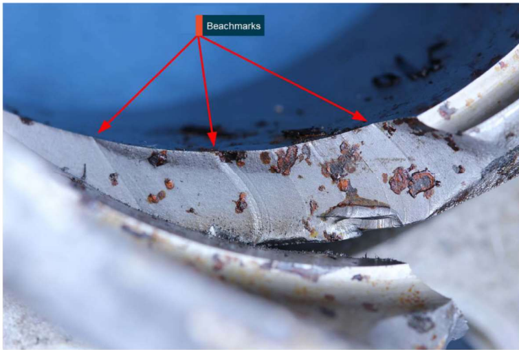
Figure 5. Image shows the progression marks on the fracture surface, which was indicative of a fatigue failure mechanism. Source: ATSB
