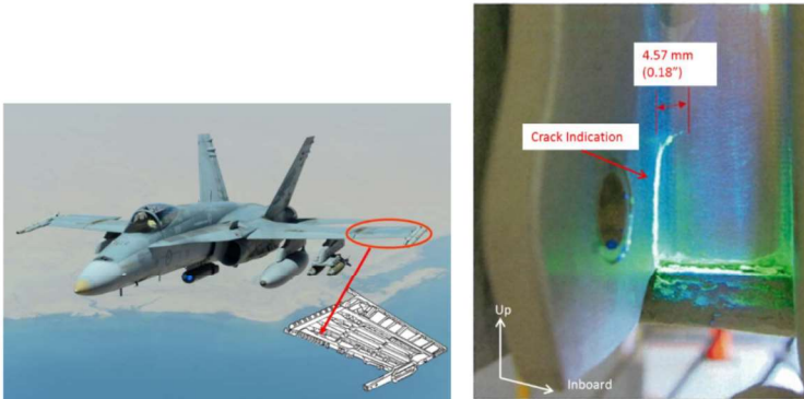
Figure 1. The outer wing of the F/A-18A/B Hornet with the location of the OLEF Hinge Lugs marked (left) and (right) liquid penetrant indications of fatigue crack growth from an in-service outer wing exhibiting MID.
