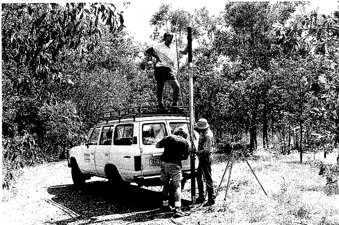
FIGURE 5.9 Various methods of obtaining water samples were used. Here a double packer (black sections at each end) pump system is being prepared for lowering down PH15 on Section 6048 mN. Work was mostly done during the “dry” season – the dry brown “spear” grass attests to the intense seasonal aridity and high temperatures (around 35°C).
