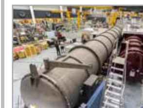
Small Angle Neutron Scattering (SANS) instruments Quokka (left) and Bilby (right) at ANSTO used to quantify the nanoscale precipitation in structural alloys.
