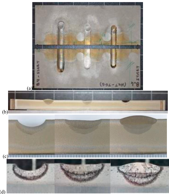
Fig. 4. (a) The trial three-slot specimen filled with a single, two and three weld passes after the performed EDM contour cut and (b) a view of the transverse-normal plane after cutting. (c) The three slices extracted from one half and (d) the macrographs acquired after chemical etching of the samples.
