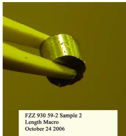
Figure 2. As-Machined fuel core specimen cut from mini-element 59-2.
