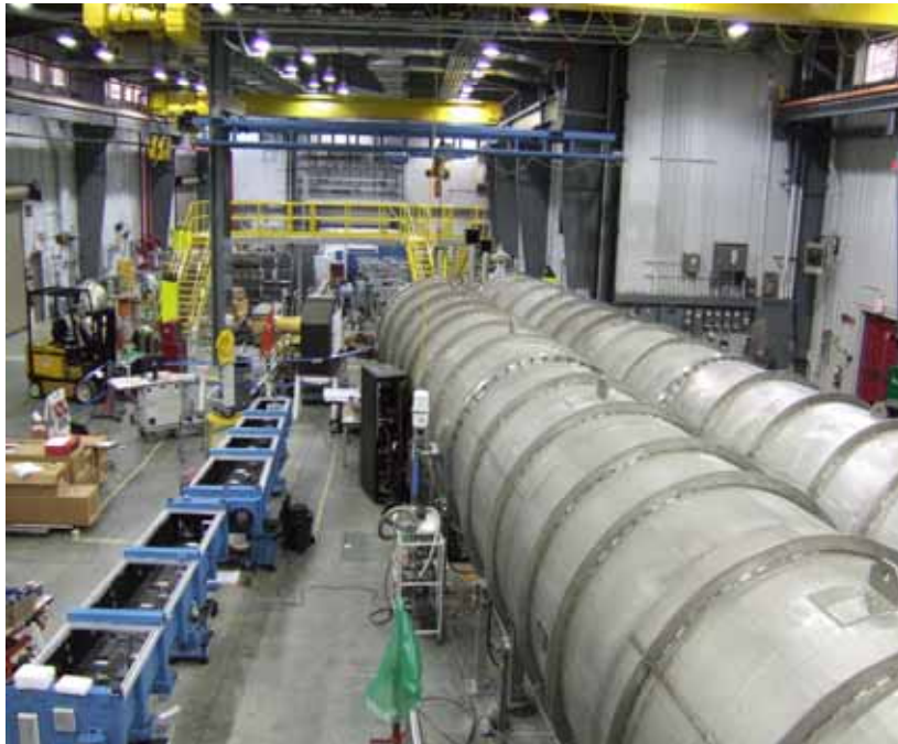
Figure 5: SANS-1 and SANS-2 Flight Tubes
