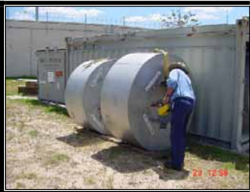
Cask Survey prior to setting up casks
