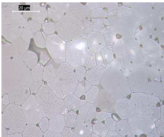
Figure 8-1. Micrograph of the polycrystalline as-polished sample of In-doped TiO 2
