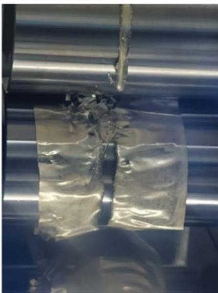
Figure S8. Optical photos of lithium strips (rolling to 40 \mu\text{m} ) during actual processing. (a) No ZDDP was used for rolling
