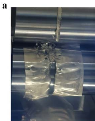
Figure S8. Optical photos of lithium strips (rolling to 40 \mu\text{m} ) during actual processing.
