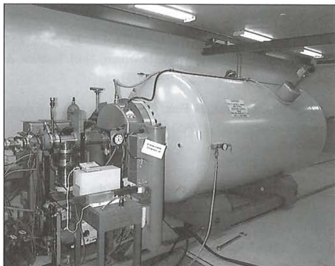
Fig. 1. 3 MV Van de Graaff accelerator. The accelerating tube and high voltage components are housed within the tank, which is pressurised with a mixture of \text{CO}_2 and \text{N}_2 for electrical insulation.
