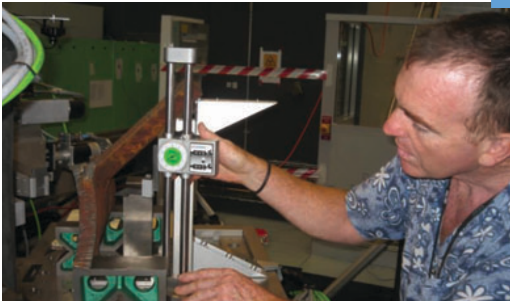
Figure 2 - Positioning a section cut from the branch connection on Kowari.
