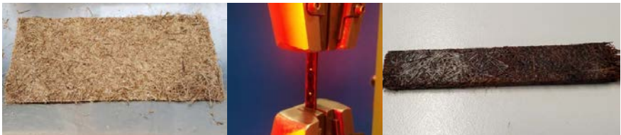
Figure 1. (Left) Harakeke Fibre Mat Production, Figure 2 (Centre) Neat Furan Matrix Tensile Testing, Figure 3 (right) Bio- Composite Preparation
