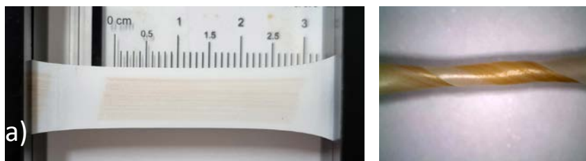
Figure 1. Stretching (a) and twisting (b) of inkjet printed PEDOT-g-PAU
