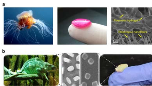
Figure 1. Electrospun nanofiber and hydrogel-based nanostructured smart biomaterials inspired by (a) jellyfish mesoglea and (b) chameleon skin.
