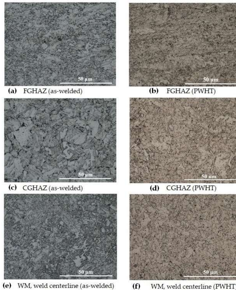
Figure 8. Optical micrographs showing the FGHAZ, CGHAZ, and the WM in the as-welded (a,c,e) and after PWHT (b,d,f) specimens .
